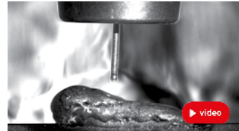
CMT WITH SCHLIEREN IMAGING (CAVILUX HF AND SMART)
