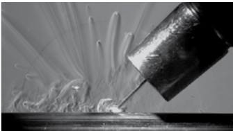
SCHLIEREN IMAGING OF ARC WELDING - WITH FRONT-ILLUMINATION (CAVILUX HF)
