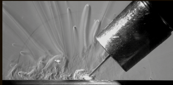
Schlieren imaging of arc welding – With front-illumination
