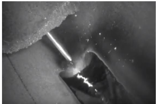
Direct illumination of tee-joint arc welding from front
