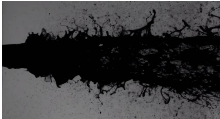
Figure 1: Spray of fuel oil captured at 20.000 fps. Use of an effervescent nozzle. Field of view of 5 mm x 20 mm
