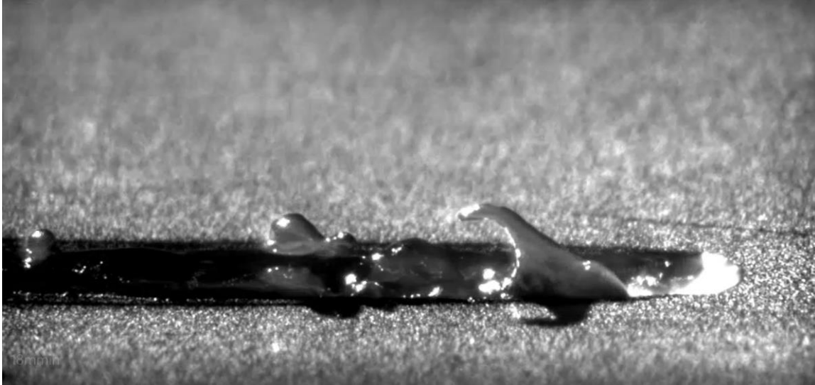
Image 1: Formation of capillary in melt pool of laser welding. Captured at 20.000 fps.
