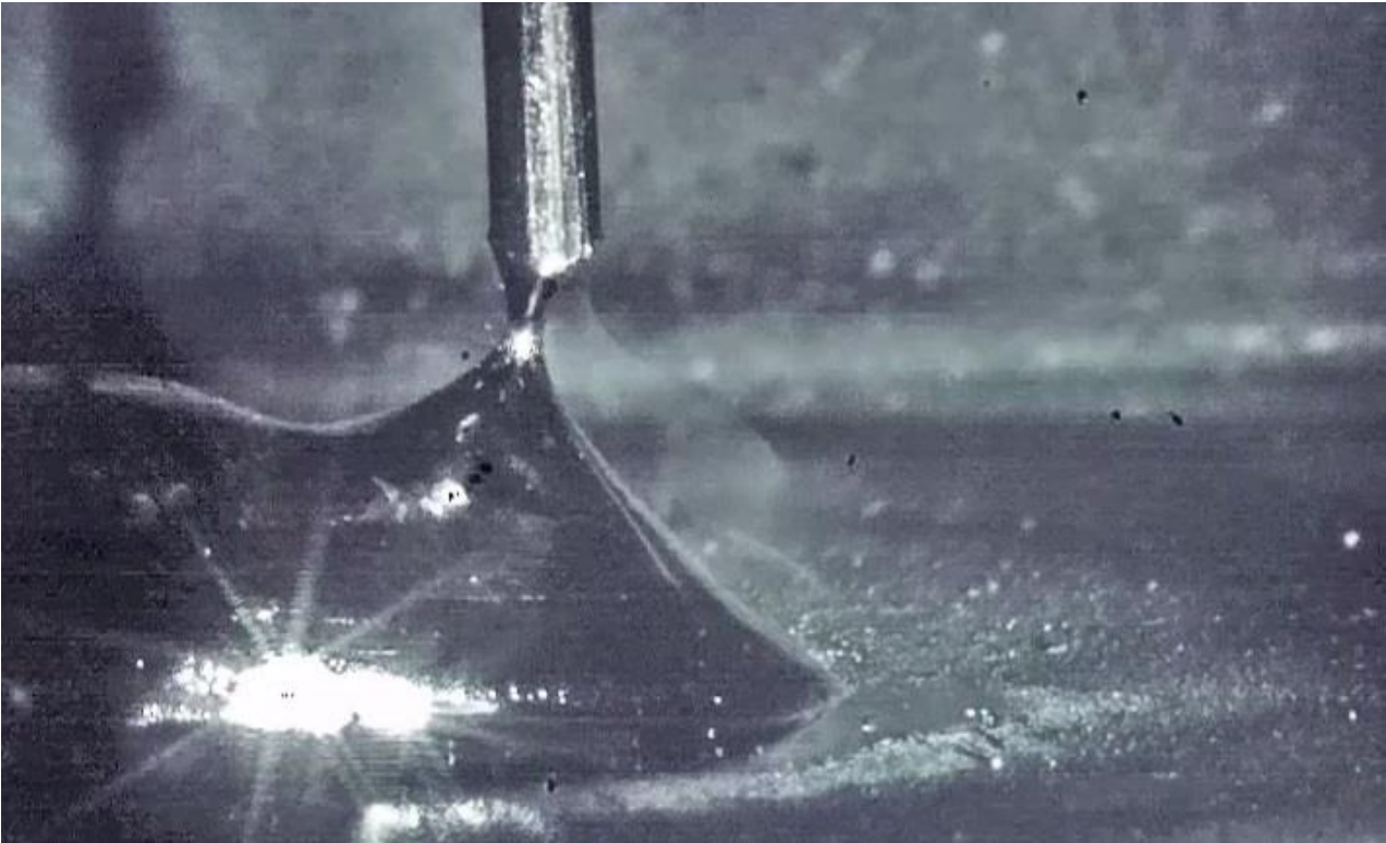
Figure 3: MIG/MAG Welding with forward/backward movement of the wire electrode imaged at 4.166 fps
