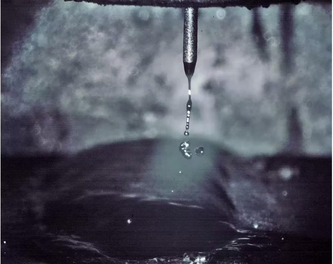
Figure 2: Rotary Arc Pulsed MIG/MAG Welding imaged at 5.000 fps
