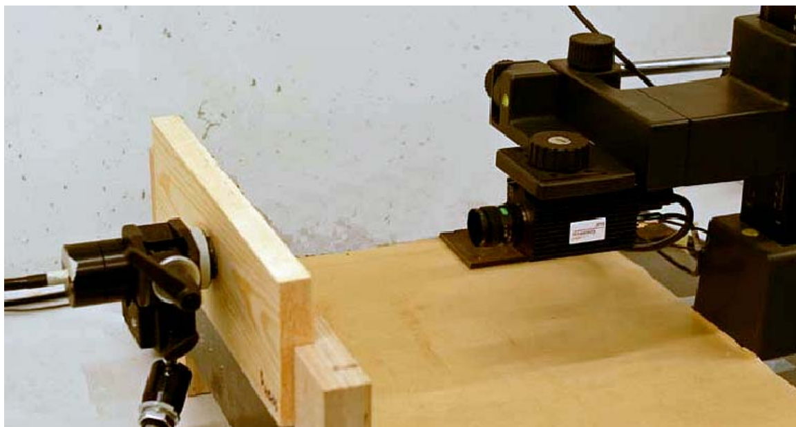
Figure 1. Measurement setup for the transillumination of wood.
